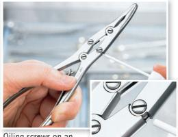
Oiling screws on an articulated instrument
